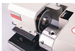
Cutting carbide end mill performance \varnothing 10 end mill takes approx. 55 seconds \varnothing 16 end mill takes approx. 100 seconds
