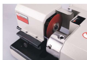
Cutting HSS end mill performance \varnothing 10 end mill takes approx. 60 seconds \varnothing 16 end mill takes approx. 110 seconds
