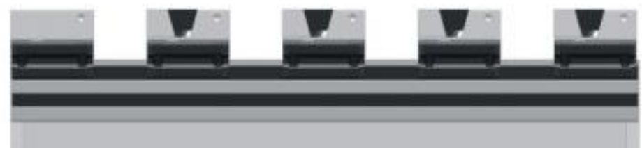
基座垂直於機台 Alignment with perpendicularity setup.
